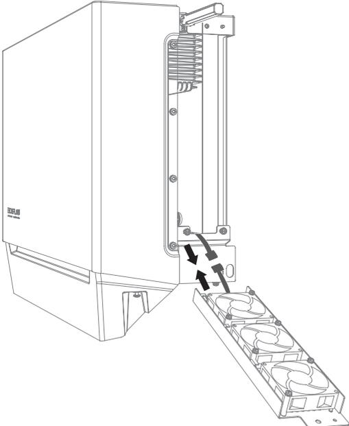
4. Secure the bottom screws, and lower the handle.
