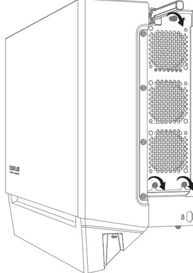
1. Prepare a new fan and install it on the inverter. To install a new fan:
