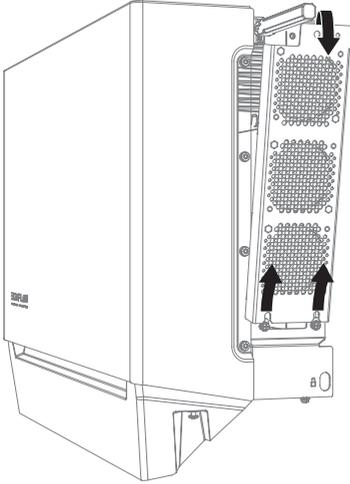
2. Align the locating pins and place the fan module into the fan position.
