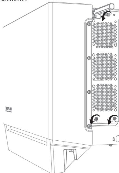
3. Pull the top screw by hand to remove the fan module.
