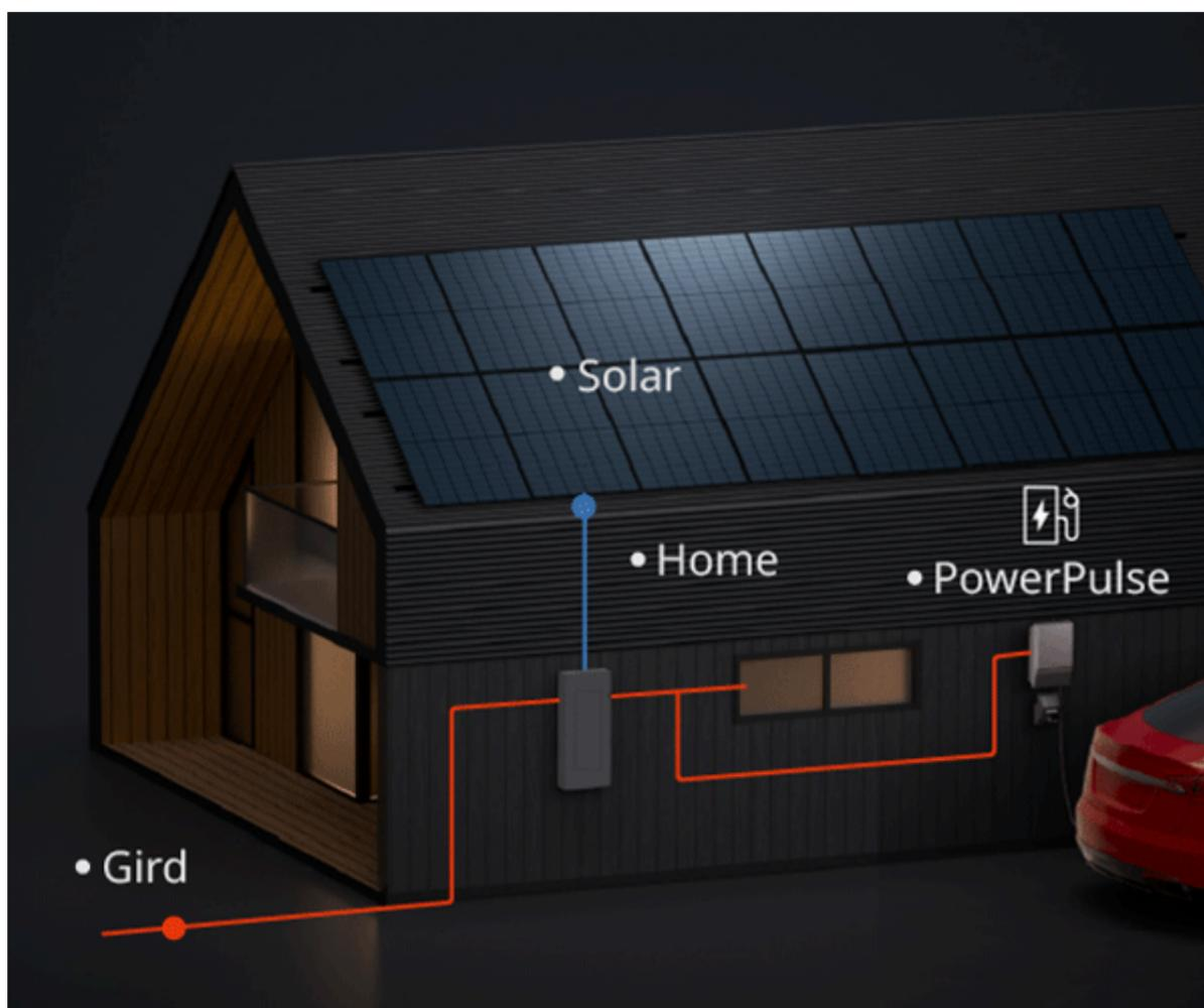
When using it, you can choose custom, fast charging or solar charging mode in the EcoFlow app. After selecting the solar charging mode, the EV charger will draw power from solar energy first. When the real-time solar energy input is not enough to maintain the minimum power of the EV charger (single-phase 1.38kW and three-phase 4.2kW), the EV charger will draw power from the grid to ensure that the charging current remains  $\geq 6A$  to maintain the normal operation of the EV charger.
