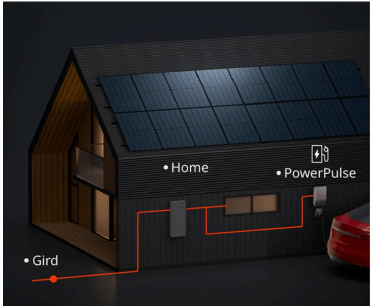
After the load balancing function is turned on, please set the maximum load current of the household according to the main circuit breaker parameters. The product will read the real-time load current of the smart meter and always intelligently charge the car with the maximum current allowed by the system ( $\leq 16A$ ). While maintaining fast charging, it also maintains the stability of circuit operation.
