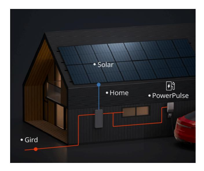
When using it, you can choose custom, fast charging or solar charging mode in the EcoFlow app. After selecting the solar charging mode, the EV charger will draw power from solar energy first. When the real-time solar energy input is not enough to maintain the minimum power of the EV charger (single-phase 1.38kW and three-phase 4.2kW), the EV charger will draw power from the grid to ensure that the charging current remains ≥ 6A to maintain the normal operation of the EV charger.
